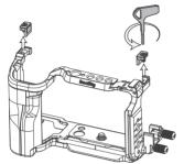
Step 1: Put the camera into the cage from back to the front. 第一步: 将相机从后往前放入拓展框。
