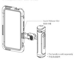
3. Quick Release: There is a Quick Release Slot on each of the four sides of the cage frame. The Quick Release Slot interfaces with the 1/4"-20 threaded holes on the cage, expanding SmallRig's unique Quick Release Ecosystem.
