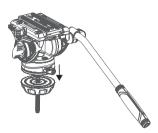
2. Tighten the screws at the bottom of the Half Ball Base
