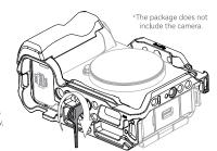
③ Use the Dual-Head Wrench to secure the bottom 1/4"-20 screw, but do not fully lock it.
