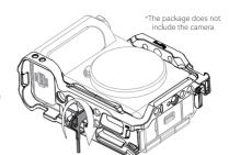
⑤ Use the Dual-Head Wrench to lock the bottom 1/4"-20 screw.
