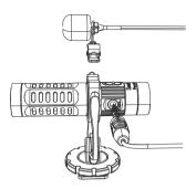
5. For the professional stereo effects, please connect a extra microphone like the customized lavalier microphone to the \$20 and toggling the mode switch button to "S" mode. In this manner, you can obtain a stereo sound which is more suitable for interview purpose.
