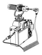
4.Connect the 3.5mm output jack of S20 with the 3.5mm input jack of DSLB camera via the 3.5mm TBS cable.
