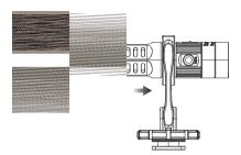
3.Putting a furry windscreen or a foam windscreen onto S20 can effectively eliminate wind noise based on recording scene needs.
