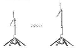
6. Expand the phone clamp, place the phone inside, and clamp it. 拉开手机夹、将手机放入并夹紧。
