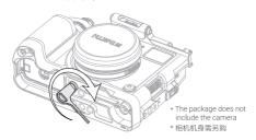
Step2: Loosen the screw, push the locating block upward toward the shoulder strap slot, and tighten the screw.
