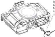
Step 2: Lock and install the cage via tightening the 1/4"–20 screw on the bottom.
