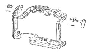
Step1: Put the camera into the cage from back to the front.
