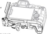
Step2: Stretch the side plate outward and lock the bottom 1/4"-20 screw.
