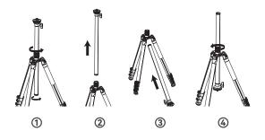
Adjusting the Integrated Levelling Base
