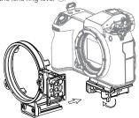
\*The package does not include the camera. Adjust the position of the lens ring to align with the center of the lens, and then use the allen wrench to lock it.
