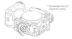
5. Use the Allen Wrench to lock the M2.5 screw removed in step 2 through the left shoulder strap hook hole to the cage.
