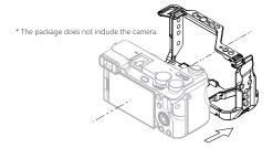
3. Use the Dual-Head Wrench to lock the bottom 1/4"-20 screw.
