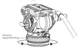
Unlock the Pan Locking Lever for 360° panning.
